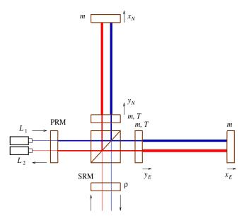
FIG. 1 (color online). Scheme of an Advanced LIGO interferometer pumped by two lasers. The main laser is detuned to give a positive optical rigidity and negative damping (it is tuned on the right slope of resonance curve), while the auxiliary laser is detuned to give negative optical rigidity and positive damping.
